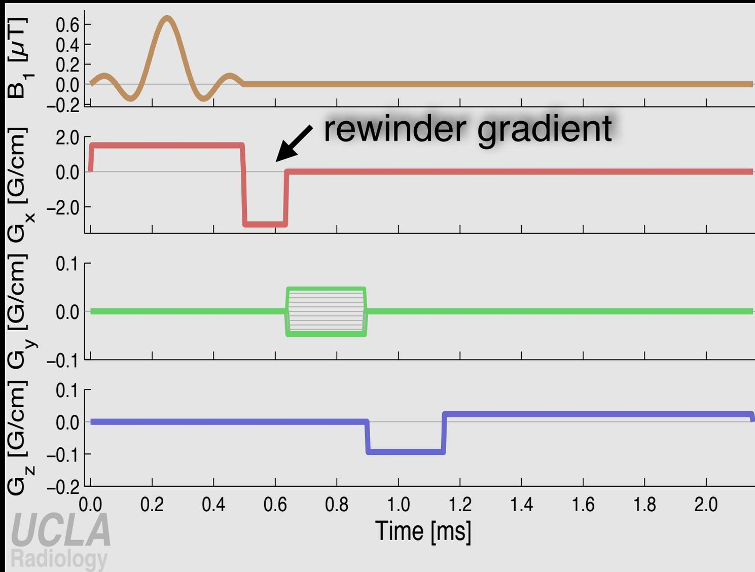
slice select gradient rewinder eliminates the linear phase ramp
